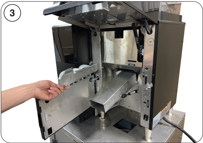
3 Move the swing arm to the side and use a tool to hold into place (optional).
