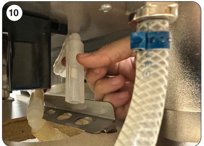
10. Remove the drain fittings from the bracket.
