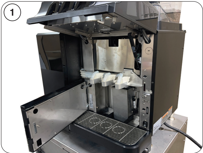
1 Power off the machine and open the lower and upper door.
