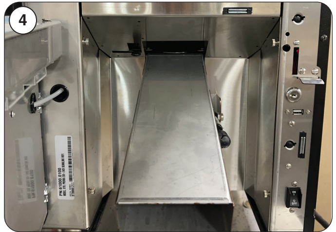
4 Remove the four thumbscrews that secure the shroud to the machine.
