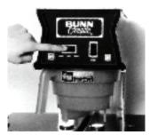
Place the power switch in the ON position (Model TL3) or select the desired reservoir RIGHT or LEFT (Model TL6).
