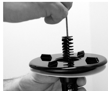
9. Clean the inlet tube with the medium sized brush and the cleaning solution.
