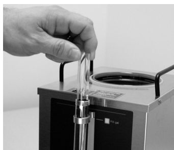
12. Remove the glass tube.
