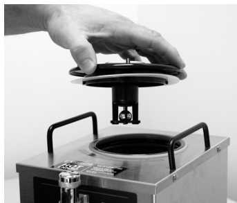
7. Pull out the lid assembly.
